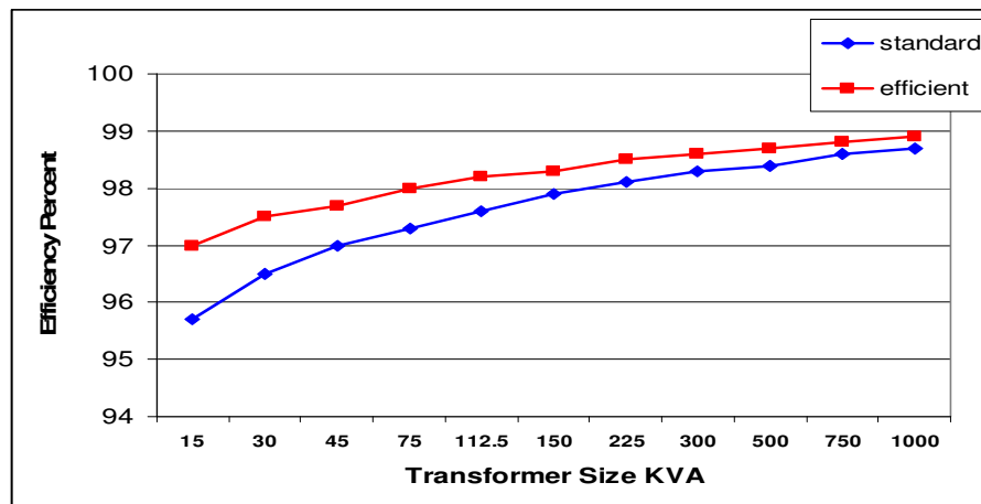
Figure 32. Transformer Efficiency Specification NEMA TP-1
